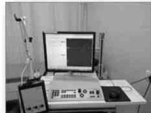
Fig. 1: The Electromyograph. The equipment used in EDx essentially consists of a computer with a stimulating apparatus a head-box to collect the biological signals from the patient and a loud speaker to listen to the EMG signal
